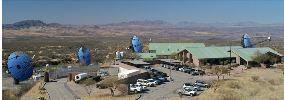
VERITAS Arizona, USA 1275m a.s.l. 4 telescopes, \varnothing 12\text{m} Stereoscopy >2007
